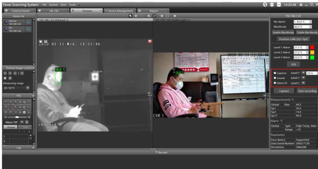
Figure 10 Alarm event (image capture and sound alarm)
